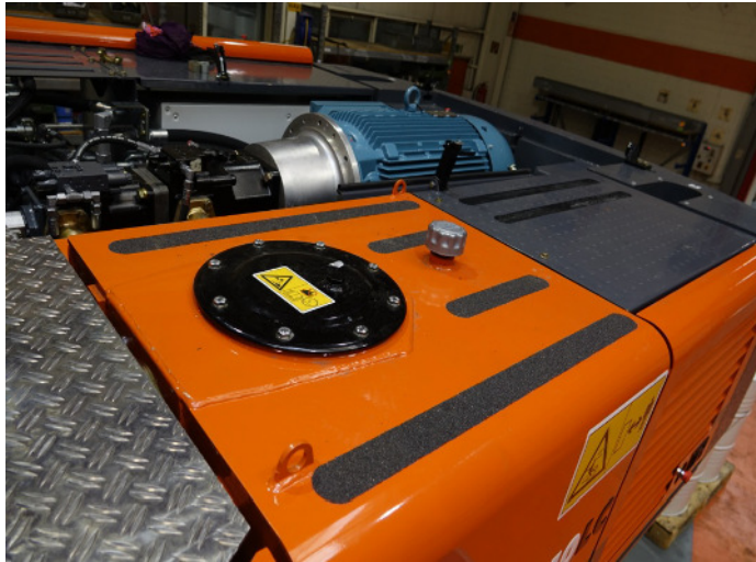
Powerful 132KW electric engine at ATLAS 340LC / 350 MH. (optionally 90 kW)
