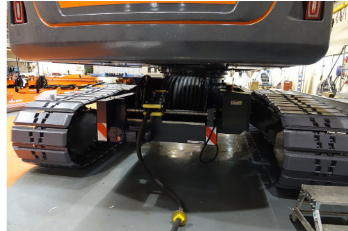
Compact electric cable drum at 340 LC with 60 meter cable. Proportional moving to machine speed.
