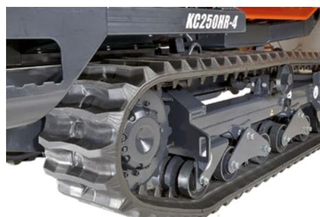
The KC250-4 track mechanism features triple flange rollers. 8 track rollers are mounted on bogey type technology, it ensures great stability on slopes and rough terrain. The short pitch track offers smooth drive for an optimal comfort at high speed.
