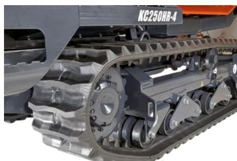
The KC250-4 track mechanism features tripple flange rollers. 8 track rollers are mounted on bogey type technology, it ensures great stability on slopes and rough terrain. The short pitch track offers smooth drive for an optimal comfort at high speed.
